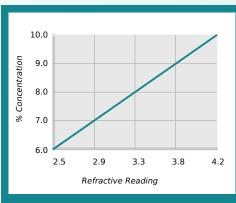
% Concentration = Refractive Reading x Refractive Factor Coolant Refractometer Factor % Brix = 2.4
