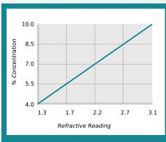
% Concentration = Refractive Reading x Refractive Factor Coolant Refractometer Factor % Brix = 3.2
