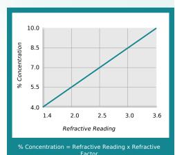
Coolant Refractometer Factor % Brix = 2.8
