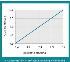
6 Concentration = Refractive Reading x Refractive Factor Coolant Refractometer Factor % Brix = 2.9
